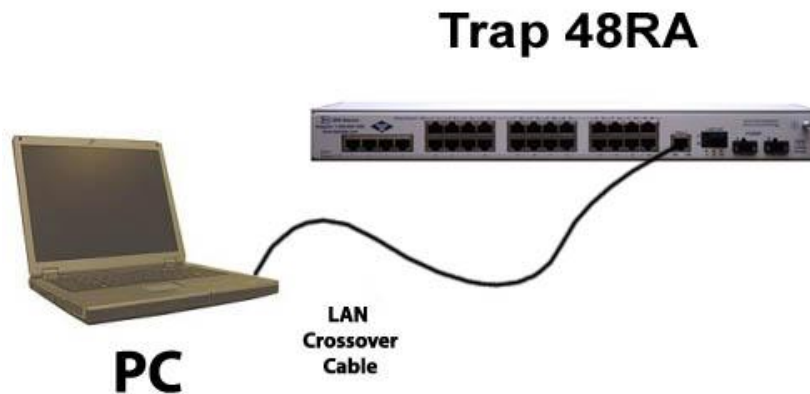
Fig 7.2 Connection through Ethernet port
