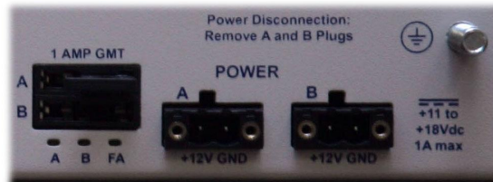
Fig. 5.2 The Trap48 RA's power inputs
