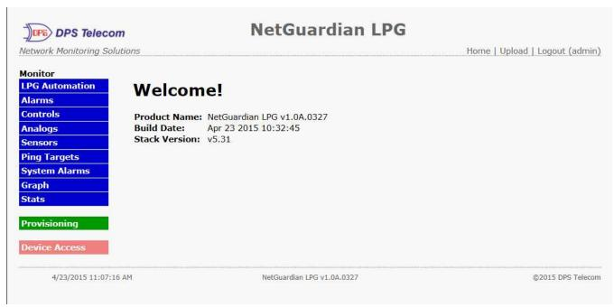
To upload firmware, click on Upload on the top right corner of the web interface
