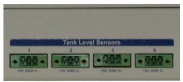
The Tank Level Sensor Inputs on the NetGuardian LPG Controller.
