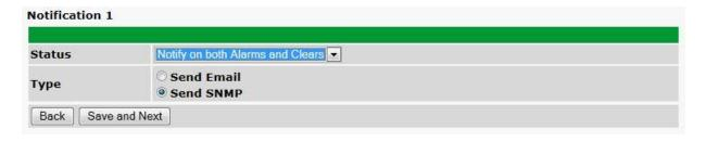
4. At the **SNMP Notification** screen, you'll enter your network's SNMP settings. Enter the **IP address** of your SNMP Trap Server. Enter the **Trap Port Number** (usually 162) and the **Trap Community** password. Click **Save and Next**.
