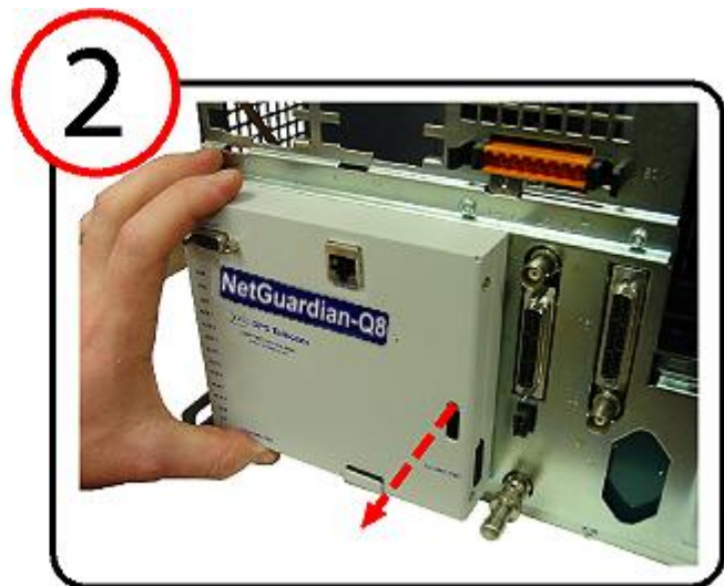
Because of its unique mounting, the NetGuardian Q-8 takes up no rack space.
