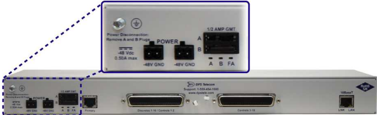
NetGuardian Power Terminals and Fuses
