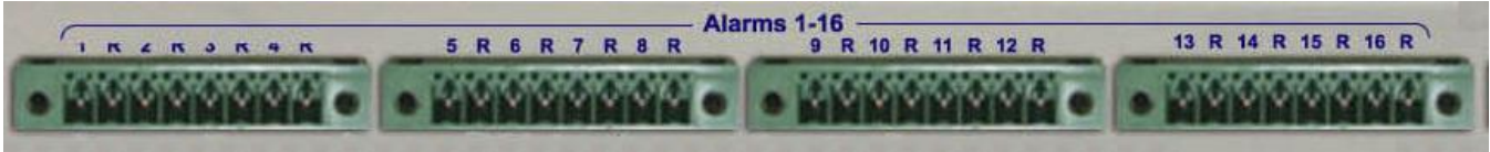
The RPS AB6's discrete alarm inputs
