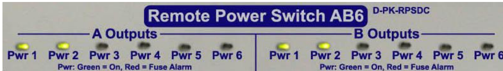
LEDs on the front panel of the RPS AB6
