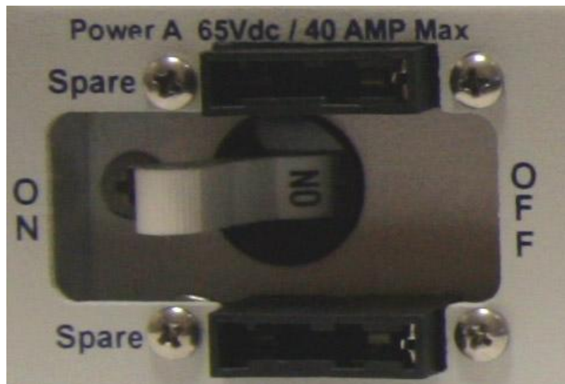
Breaker Switches are located on the front panel of the RPS AB6
