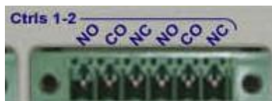
The RPS AB6's control relay inputs
