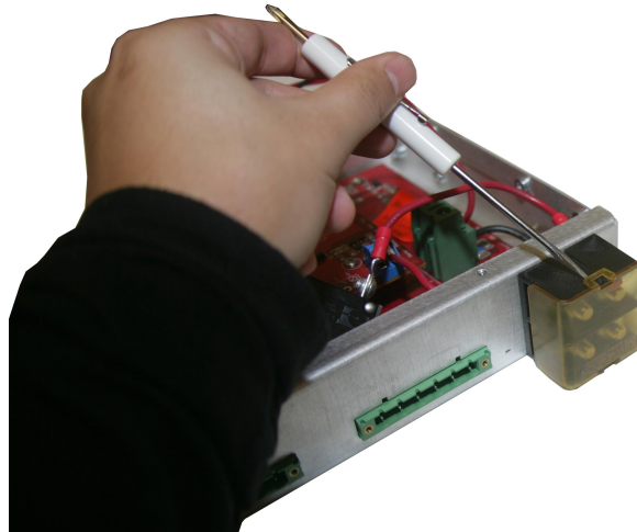
How to remove the studded power block cover
