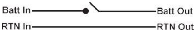
The unit's power outputs are relayed internally, allowing you to control your outputs
