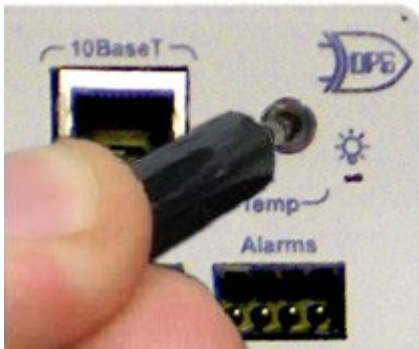
Stereo jack input on the back of the SiteMON IP G2
