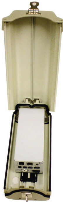
The SiteMON IP G2 inside the enclosure.
