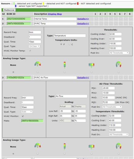
Sensor with HVAC Monitoring enabled.
