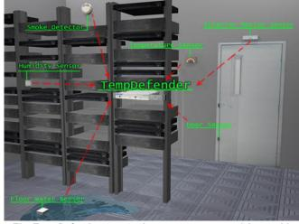
The TempDefender can monitor your server room/closet with smoke detectors, humidity sensors, floor water sensors, temperature sensors, and more.
