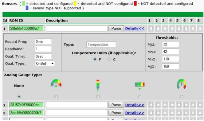
Fig. 10.22 The Provisioning > Sensors menu
