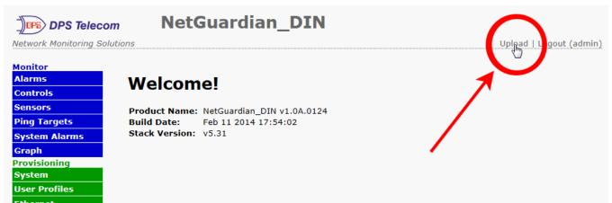
Fig. 13.2 To upload your configuration file, click on Upload on the top right corner of the web interface
