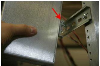
Fig. 4.1 First connect the top of the DIN clip to the rack.
