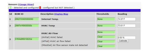
When using a Temp/Air Flow sensor for HVAC Monitoring, the HVAC Air Flow sensor monitor section will display 4 thresholds instead of one.
