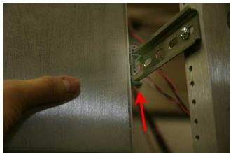
Fig. 4.2 Then snap the bottom of the DIN clip to the bottom of the rack.
