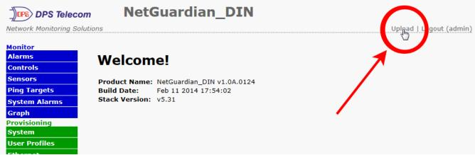
To upload firmware, click on Upload on the top right corner of the web interface
