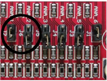
Fig. 5.3 Adjustable jumpers on the NetGuardian circuit board
