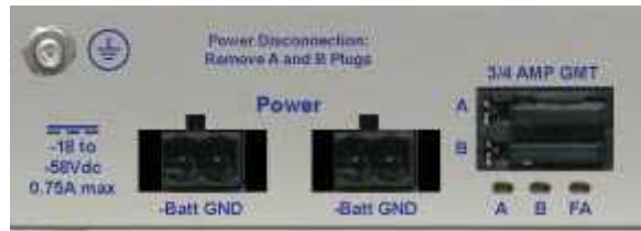
Power connectors and fuses.
