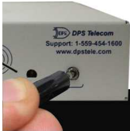
The external temperature sensor
