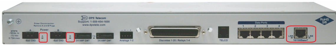
Back panel LEDs for Power (left) and Ethernet connections
