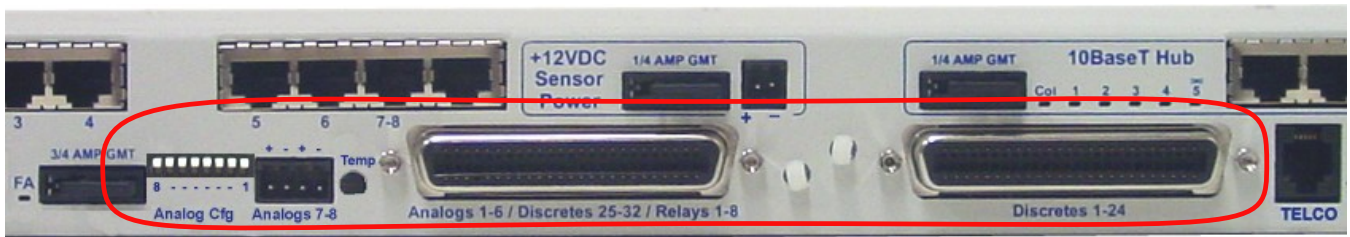
Fig. 6.6.1. Alarm and control relay connectors
