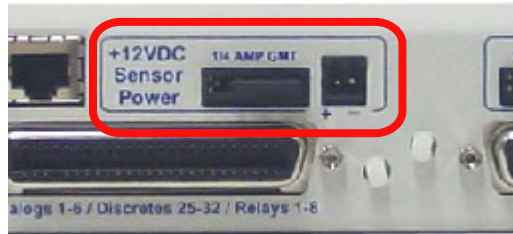
Fig. 6.9.1. +12 VDC sensor power supply
