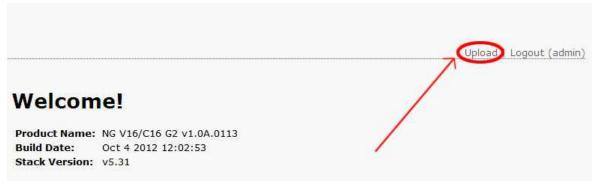
Fig. 14.1 To upload firmware, click on Upload on the top right corner of the web interface
