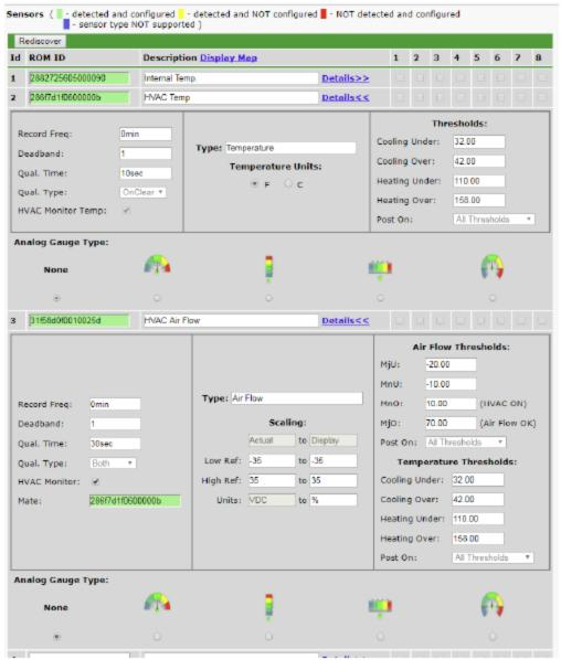
Sensor with HVAC Monitoring enabled.
