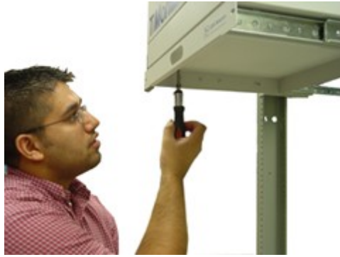
Secure T/Mon to Slide Rack
