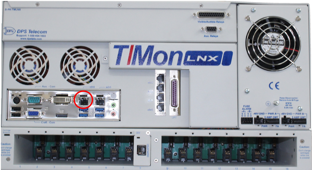
Connecting the T/Mon to LAN
